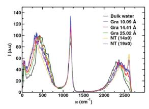
**Figure 4.** Comparison of the power spectra of the velocity–velocity autocorrelation function for all the confined water samples considered in this work. The power spectrum of bulk water is also reported for comparison.
